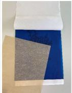
Now remove the light brown release paper between the wax foil and the white cover sheet. This cover sheet bears a colored copy of the template on the inside after the successful copying process.
